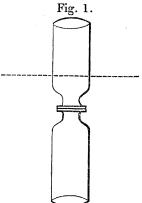
After forty-eight hours, the upper inverted bottle was again slipped off from the lower one, upon a glass plate, and the ratio of the gas found in the upper to that in the lower bottle determined by the weight of carbonate of baryta which the liquids of the two bottles afforded respectively. It was as 1.18 to 12.80 (about 1 to 11), instead of the ratio of equality, which would undoubtedly be the ultimate result of diffusion, were sufficient time allowed.
